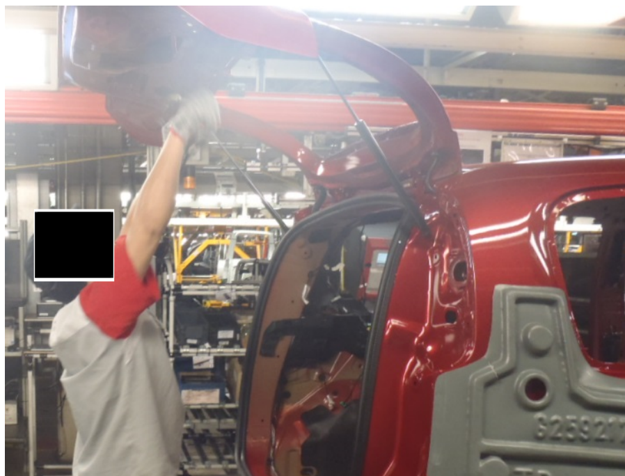
Figure 3: Tailgate wire harness assembly. Source: From authors (2018).
