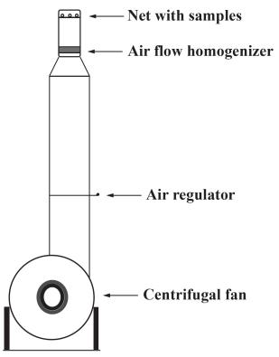
**Figure 3:** Schematic of the equipment used for measuring the terminal velocity.
