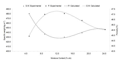
**Figure 4:** Values for porosity (%): experimental (P. Experimental) and calculated (P. Calculated), and values for specific weight (kg.m<sup>-3</sup>): experimental (S.W. Experimental) and calculated (S.W. Calculated), for each moisture content (% wb).
